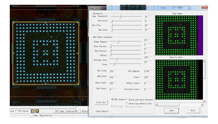
Overall inspection. Click on the "overall inspection" button to enter the overall inspection setting window. The window interface for overall inspection parameter
