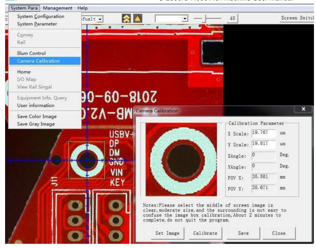
In the editing mode, select the calibration image (preferably circular mark) in the image working area by framing. In this interface, click on the "defining image" button to define the calibration image and press the "starting calibration" button to calibrate.
