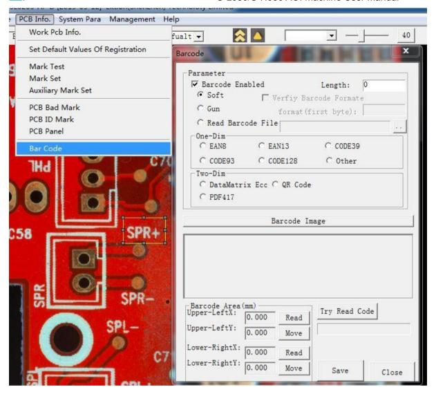
To enable the second method, bar code setting is required: select Enable Bar Code option in the bar code setting window and set the bar code length. The user can choose two different scanning modes: hand held barcode scanner and camera scanning.
