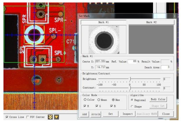
The inspection program for one PCB must set at least two Marks (it is better to find stable image features in the diagonal corners of one PCB as Mark points). Mark points will be used to correct the final positions and angles of all components to be inspected on the board, which is the basis for correct drawing and inspection of subsequent inspection algorithms.
