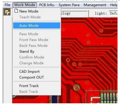
In addition to several main working modes, there is a pass mode for the on-line machine. In this mode, the boards on the track directly pass through the on-line machine. Only the number of boards is counted, and no inspection will be carried out. In other words, the on-line machine serves as a inspection conveyor.
