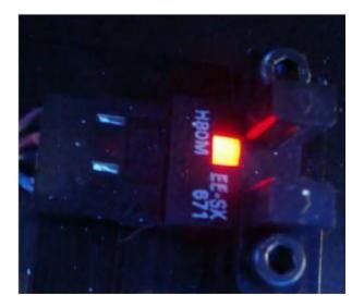
2) Determining whether the PCB photoelectric sensor works normally
