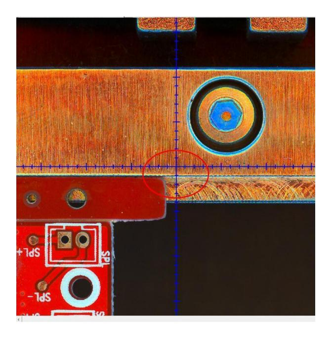
After the board size definition is completed, the operator clicks on "PCB scanning" to start scanning thumbnails of the whole board. The thumbnails will receive pixel-compression and will only play a role of position indication in subsequent operations. If the user needs to use the off-line programming (OLP), check the "saving PCB image" option before starting scanning. The image will not be
