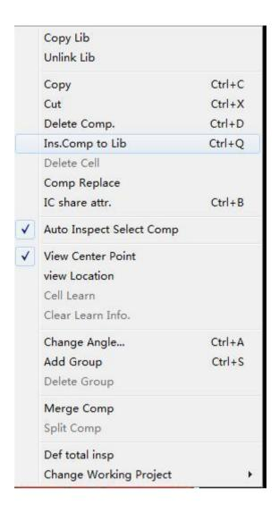
Single point copy: click this option on entered components to quickly copy registered components
