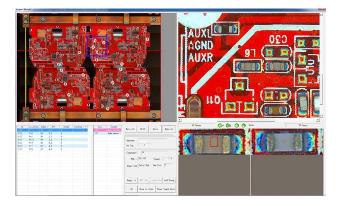
The upper right NG FOV image area displays the FOV image of the current position of NG element. The FOV image can be adjusted by scaling.
