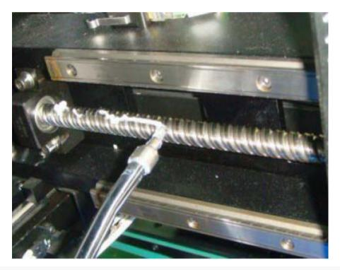
Step 3: if the slide block on the guide rail has an oil nozzle protection cover, take it off before filling.
