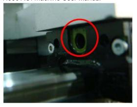
Step 4: insert the oil injection gun head into the oil injection nozzle of the sliding block and press it tightly. Gently press the pressure rod of the oil injection gun to evenly inject grease into the sliding block, and make the sliding block slide back and forth on the guide rail to evenly apply the grease.
